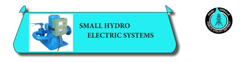
Small hydro is a hydroelectric generator on a small scale normally serving a residence, irrigation facility, a small community, or an industrial plant. The size definition of a small hydro facility varies; however, a generating capacity of up to 10 megawatts (MW) is generally accepted as the upper limit of what can be termed small hydro.
