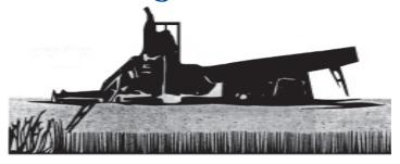
**Mechanical harvesters** are large floating machines that cut and collect aquatic plants. **Mechanical weed cutters** cut aquatic plants several feet below the water's surface but do not collect the plants while the machinery operates. Mechanical harvesters and/or cutters are not appropriate techniques to address early infestations of aquatic noxious weeds.
